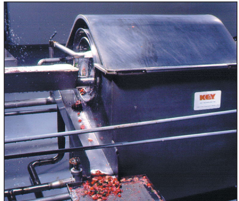
Reclaim Reel on a Strawberry Processing Line
