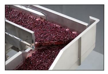
at the dryer, which needs to be fed constantly," noted Sosnicki. "And since Impulse is equipped with electromagnetic drives, we can simply adjust the speed from the control panel when needed. This makes things easier for our operators at the same time it helps preserve our product quality and increase our line efficiency."
